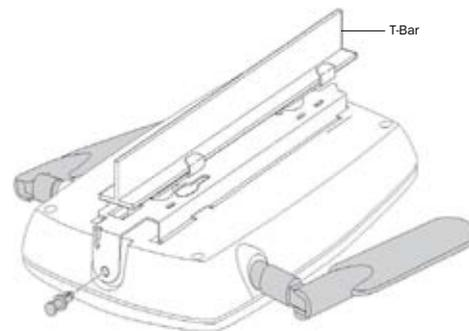
**Figure 2: Mounting Access Point to T-Bar**
